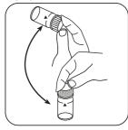
Dissolve tablet(s) by inverting.
