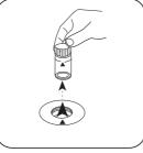
Remove the vial from the sample chamber.
