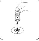
Remove the vial from the sample chamber.
